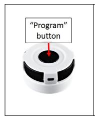
Press and hold "Program" button for 10 seconds on IR extender. The LED will flash twice until reset process is completed. Once IR extender is being "factory reset", you need to include the IR extender to the gateway again and learn the code again.
